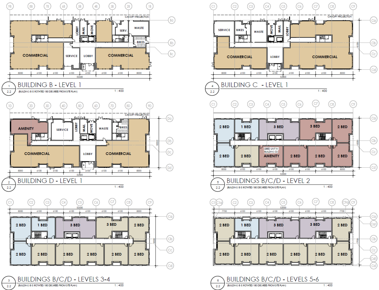
Figure 4-4: Buildings B/C/D Floor Plans
