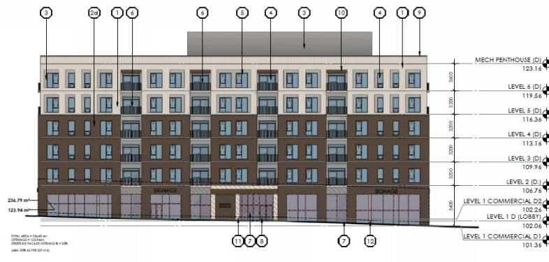
1 BUILDING D - SOUTH ELEVATION
