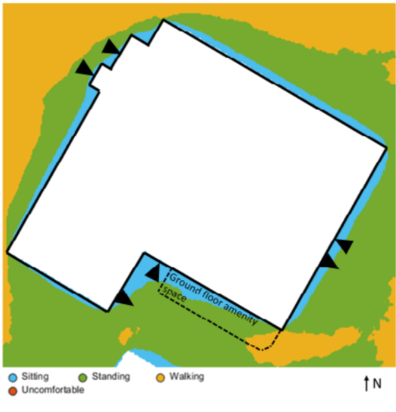
Figure 4.5 - Proposed summer wind conditions on the ground floor (left) and rooftop (right) amenity spaces (Boundary Layer Wind Tunnel Laboratory)
