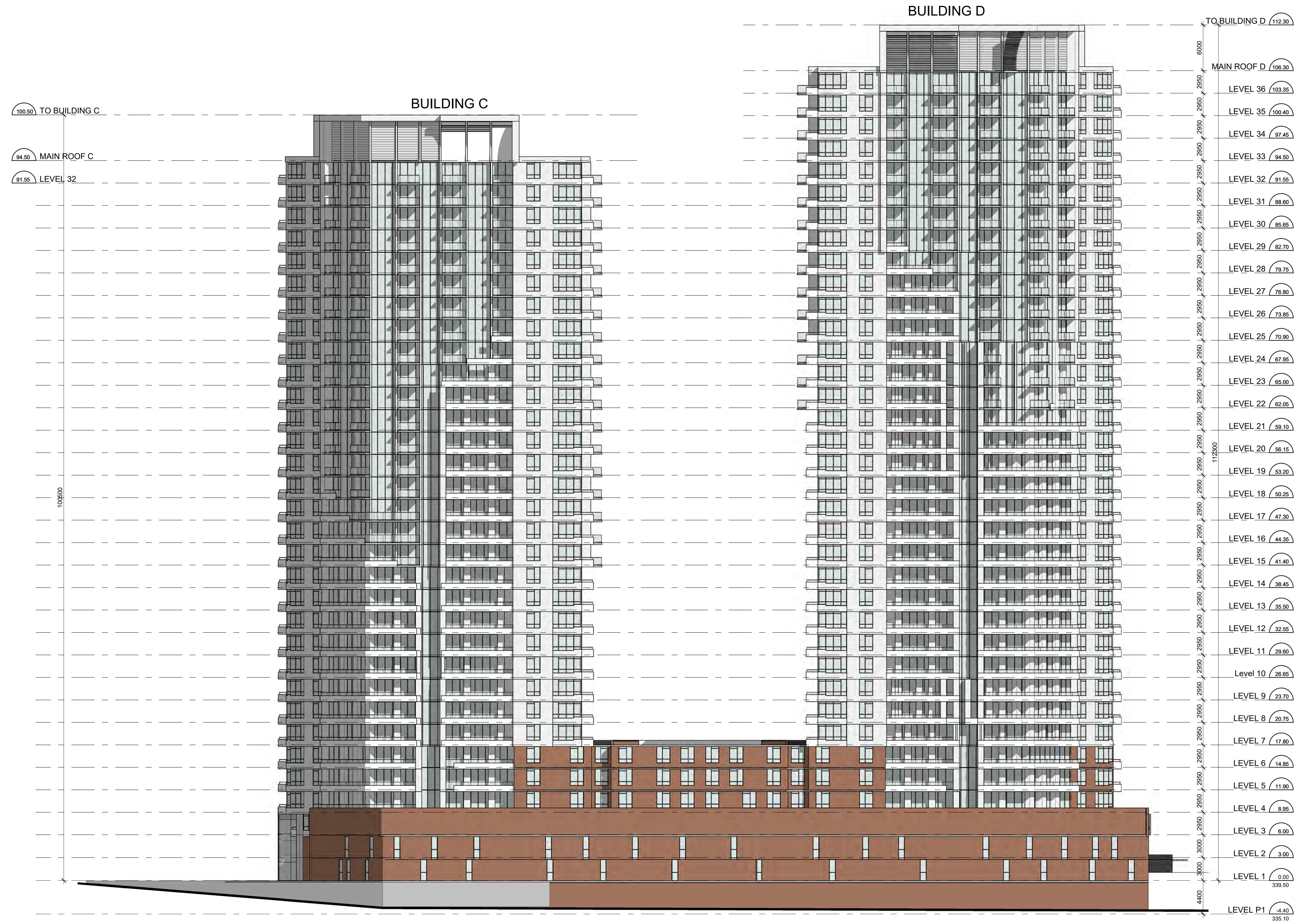
Building C & D - South Elevation 1 Scale: 1 : 250 A4.06
